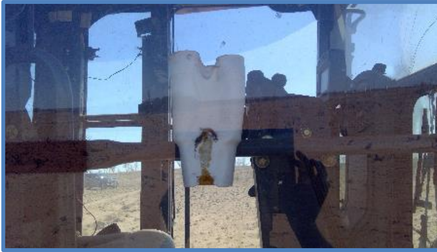
Cup melted to the inside of Alex's grader cab by radiant heat.
