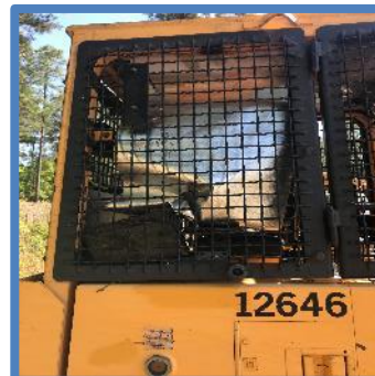
Left: Fire curtain from the inside of the cab of a tractor. Right: Fire curtain from outside the cab.
