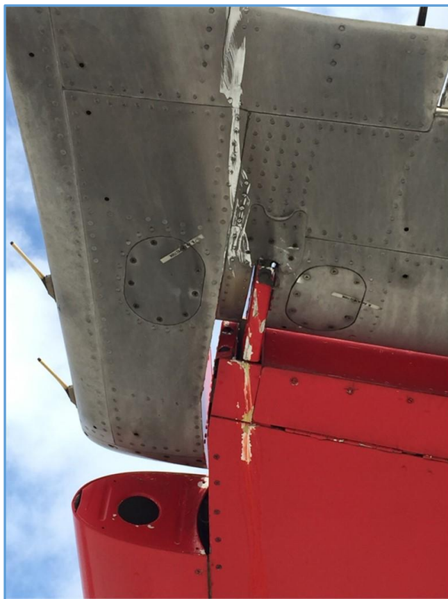
Photo shows some of the damage that occurred to the underside port wing of Tanker 41.
