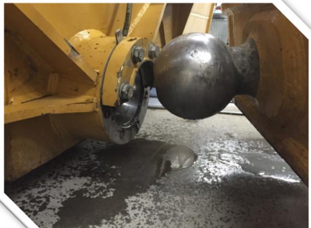
Dozer #1's trunnion ball pivot was separated from the blade.
