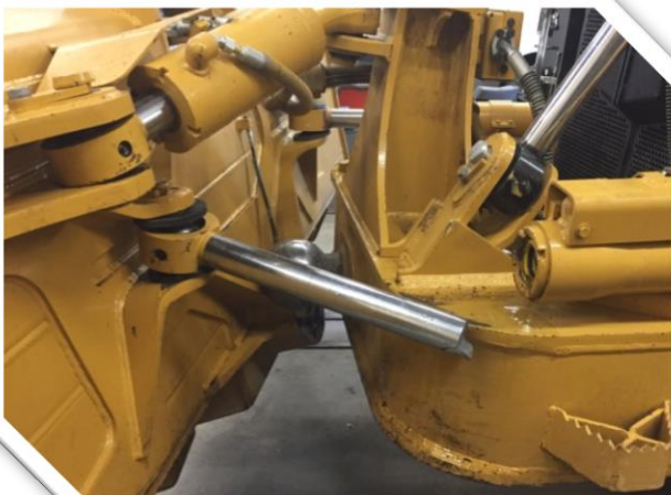
Dozer #1's left blade angle ram as well as its tilt ram were both broken.
