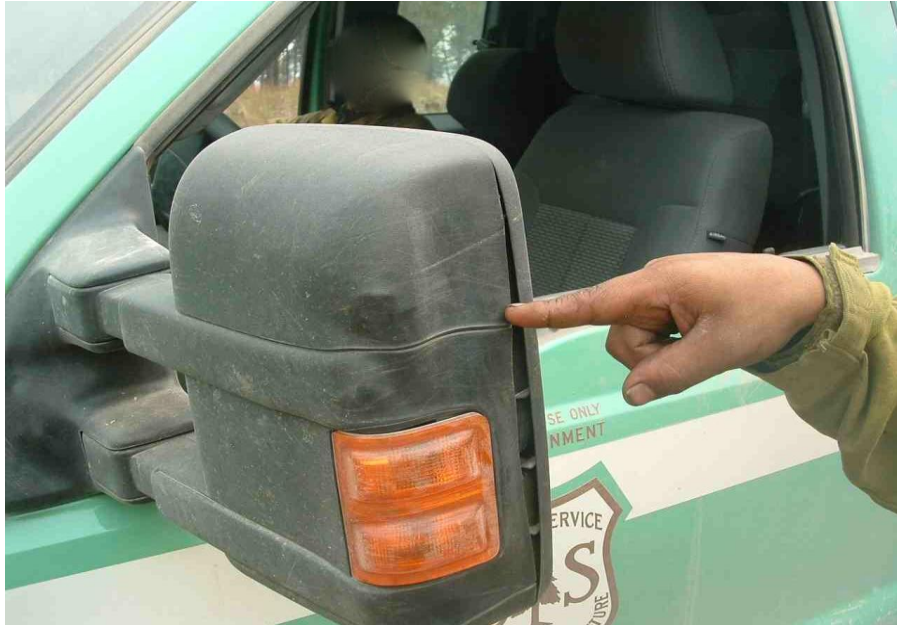
Engine 2- deformed mirror caused by radiant heat
