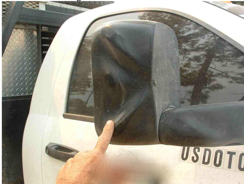
Engine 1 - deformed passenger side mirror caused by radiant heat
