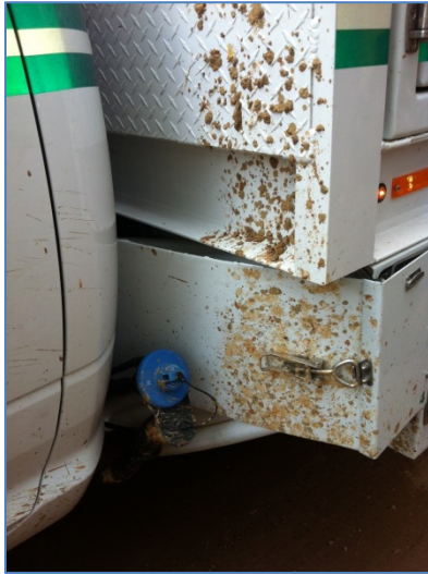
Top Photo –The pre-connect filled with water and ruptured Bin #4.
