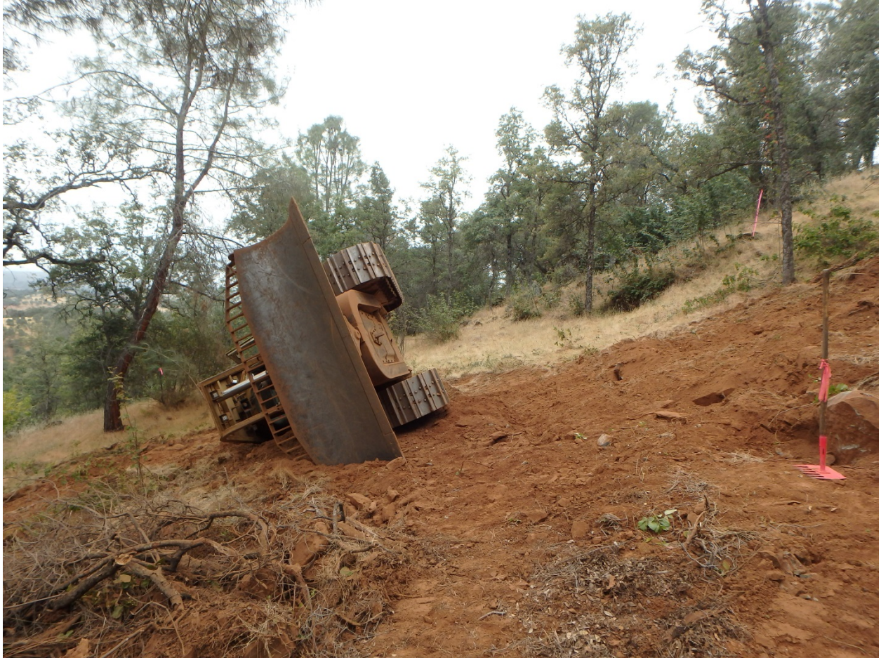
View of D3140 perpendicular to the hillslope at resting location following rollover.
