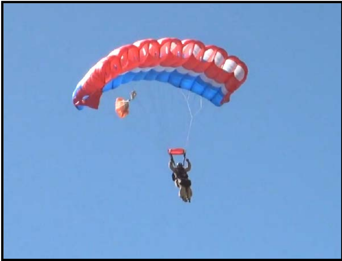
Photo 2: Jumper 6, six seconds before landing, canopy out of alignment with the wind. This image shows that Jumper 6 has turned his canopy slightly to his right.
