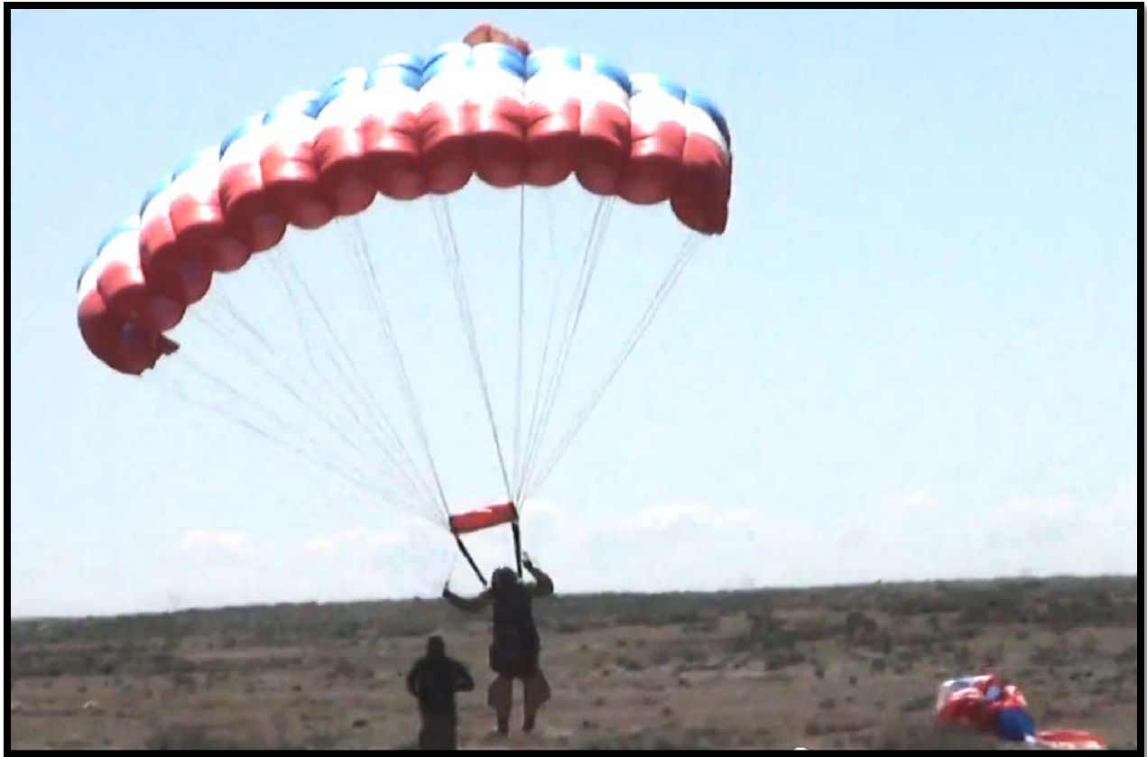
Photo 3: Jumper 6 position prior to landing. This image shows that Jumper 6's canopy is not directly in alignment to the wind.
