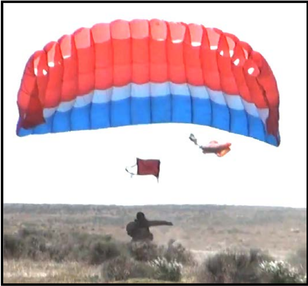
Photo 5: Main canopy is released by Jumper #6. Note cutaway accomplished with his left hand, because of damage to his right arm.
