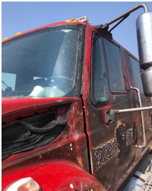
Picture shows heat damage to the engine that "blacked out" the inside of the cab.
