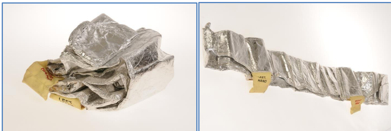
Figure 1—The deployed fire shelter as received from the Facilitated Learning Analysis Team (left), and laid out as it seemed the firefighter unfolded it at the incident (right).
