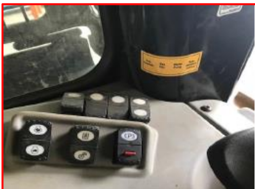
Photo shows the new parking brake switch being installed on the Cal Fire 2015 CAT D6NXL dozers. To release the parking brake after the switch is activated, the operator must depress the red locking tab then rock the switch to the “released” position. Thus, the locking mechanism on this switch will eliminate the parking brake’s accidental release. This switch change will fit all the effected Cal Fire D6NXL machines.
