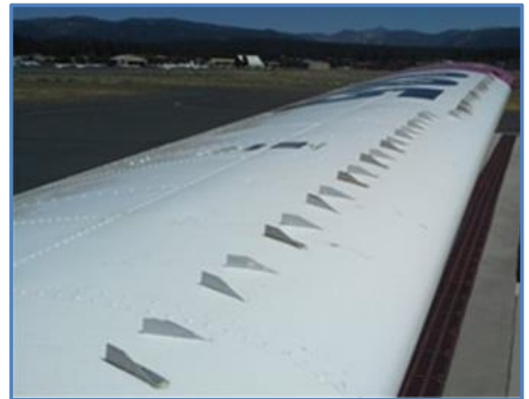
Replaced vortex generators along the aircraft's left wing. The powerline strike took out 21 of these.
