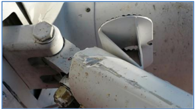
Strut damage from the wire strike with repaired step.
