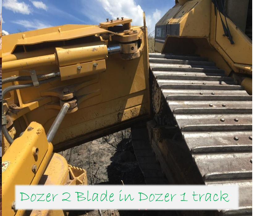
Dozer 1 damage and Dozer 2 actions to secure Dozer 1.
