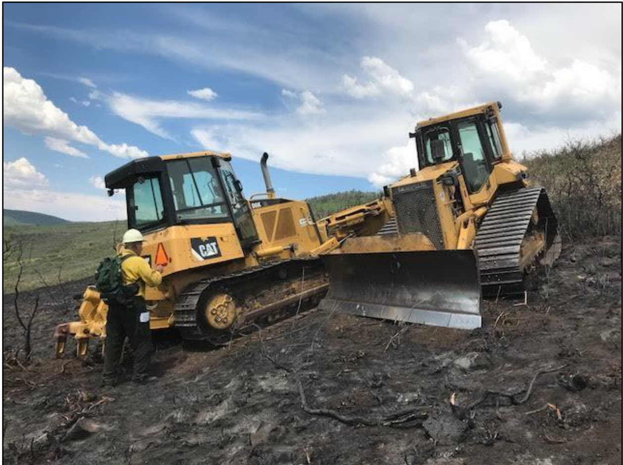
Post rollover; Dozer 2 (left) securing Dozer 1 (right).
